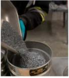
A variety of different pulverising bowls made of diverse media are available on request. All ALS equipment is standardised as low Cr-steel, however, substitution of bowls may be required when specific element contamination is a concern. Bowls available include tungsten carbide, agate and zirconium.
