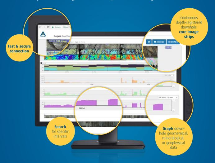
CoreViewer™ is a fast and secure core photo archive, core logging support tool, and data integration platform accessible over the web via computers and touch-screen tablets.
